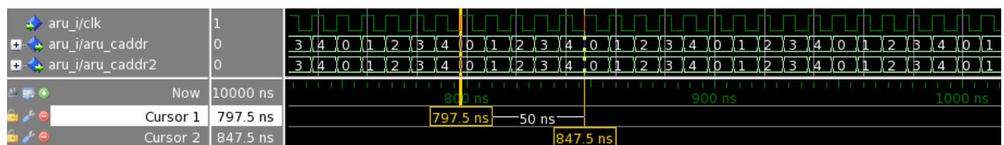
**Figure 3.4: Shortening the ARU round trip time by adding additional port to ARU**
