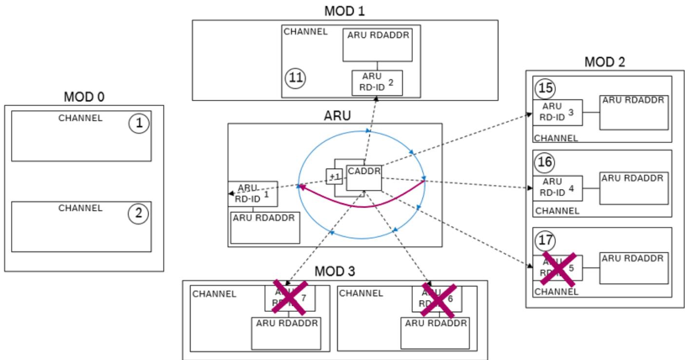
Figure 3.2: Shortening the ARU round trip time by manipulating the register **GTM.ARU.CADDR\_END**
