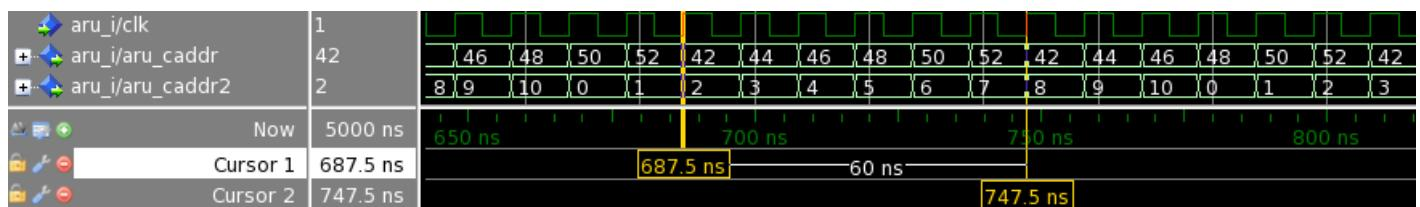
**Figure 4.10: ARU Dynamic routing, with DYN\_CLK\_WAIT=0 and ARU update mechanism disabled**
