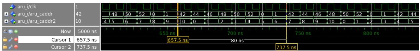
**Figure 4.11: ARU Dynamic routing, with DYN\_CLK\_WAIT=0 and ARU update mechanism enabled**
