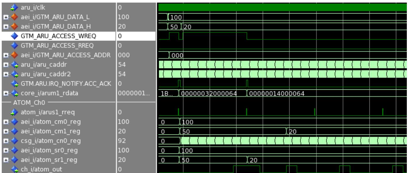
Figure 5.2: Default ARU access via CPU, CPU acts as ARU Write channel
