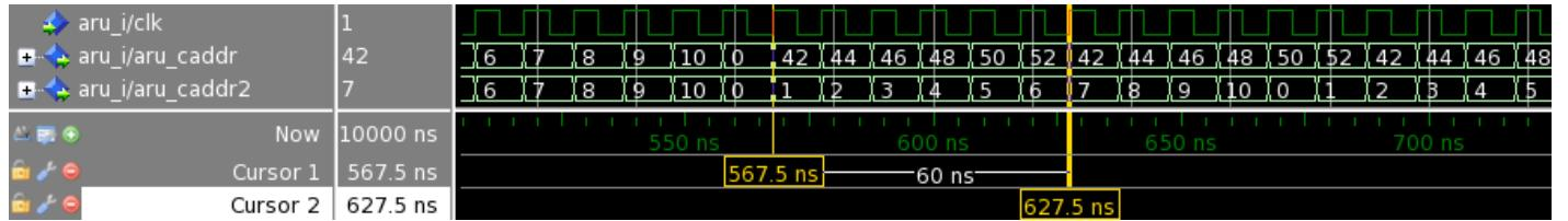
**Figure 4.1: ARU Dynamic routing: One port, DYN\_CLK\_WAIT = 0**
