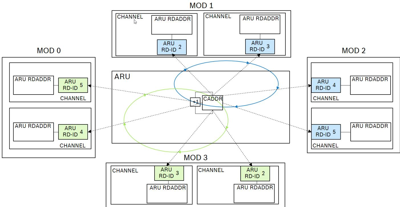
Figure 3.3: Shortening the ARU round trip time by adding additional port to ARU
