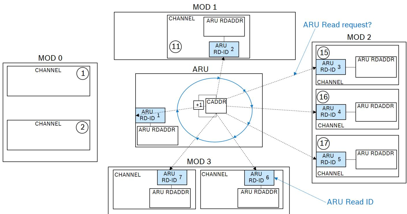
**Figure 3.1: ARU Routing scheme**
