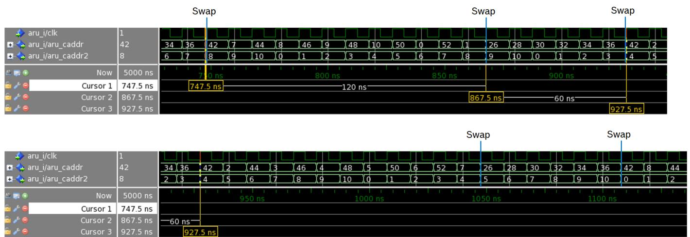
**Figure 4.6: ARU Dynamic routing, swap mechanism: One port, DYN\_CLK\_WAIT = 0, DYN\_CLK\_WAIT 1**
