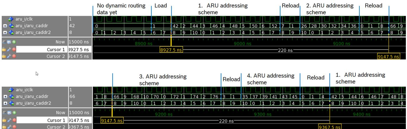
Figure 4.13: ARU Dynamic routing with ARU update mechanism via PSM
