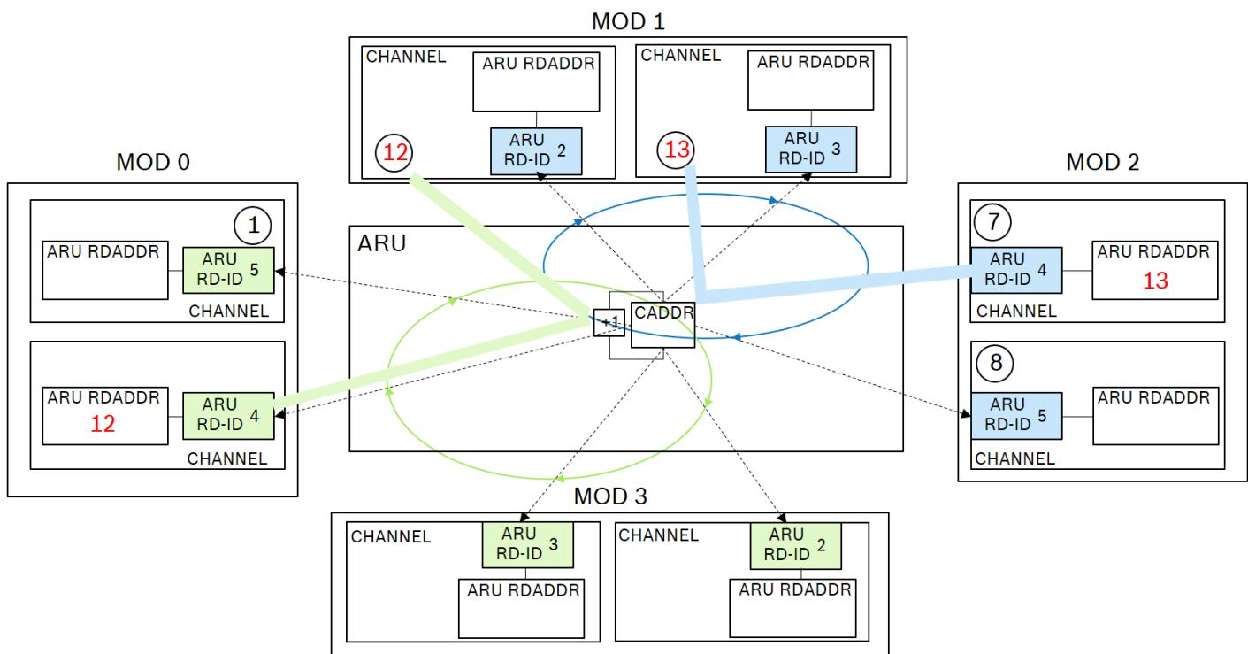
Figure 4.14: ARU data streams for two ARU ports addressing same submodule
