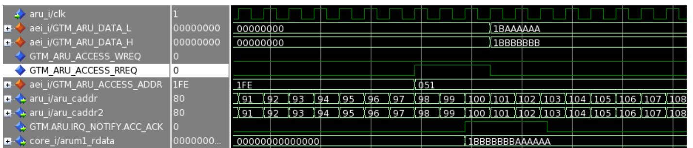
**Figure 5.1: Default ARU access via CPU, CPU acts as ARU Read channel**
