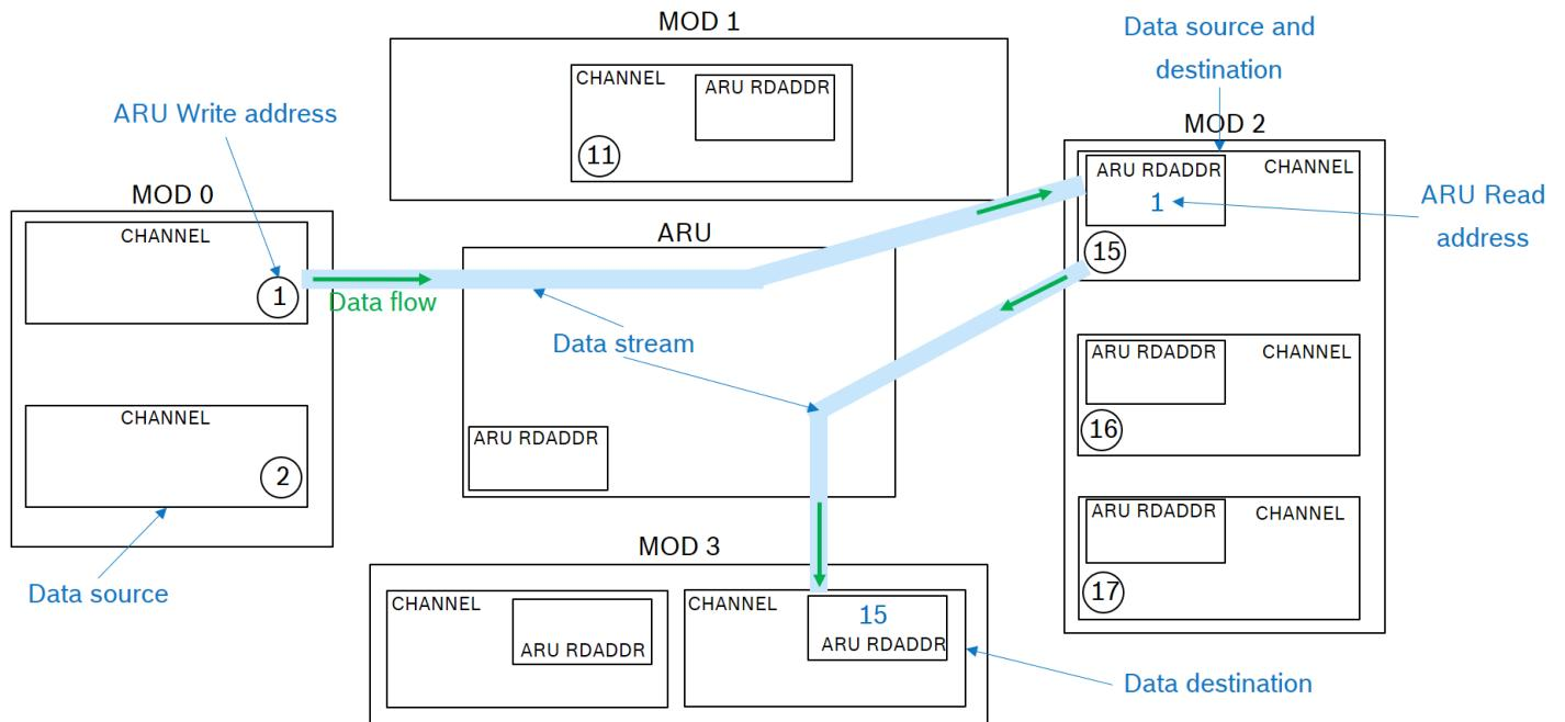
Figure 2.2: Example for ARU Routing mechanism
