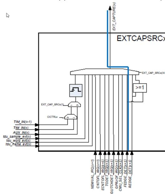
Figure 3.14: Signal path through EXTCAPSRC for falling edge propagation
