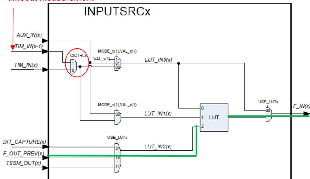
Figure 3.16: INPUTSRC configuration for TIM channel x+1 to route through the TIM channel x input signal
