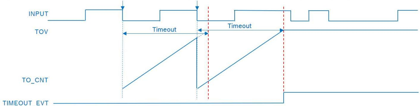
**Figure 1.2: Timeout detection for individual edges (falling to falling edge)**
