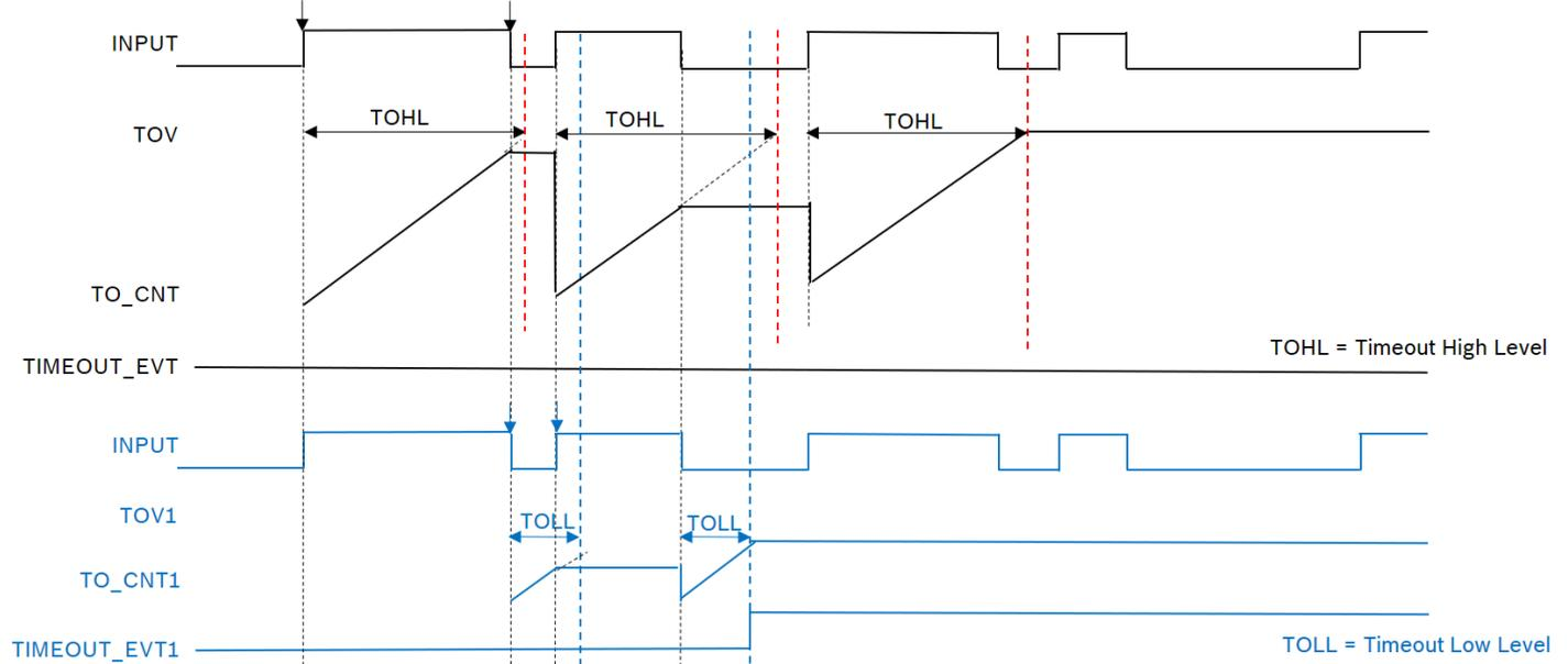
**Figure 1.4: Timeout detection for both edges (individual value for TOV and TOV1)**
