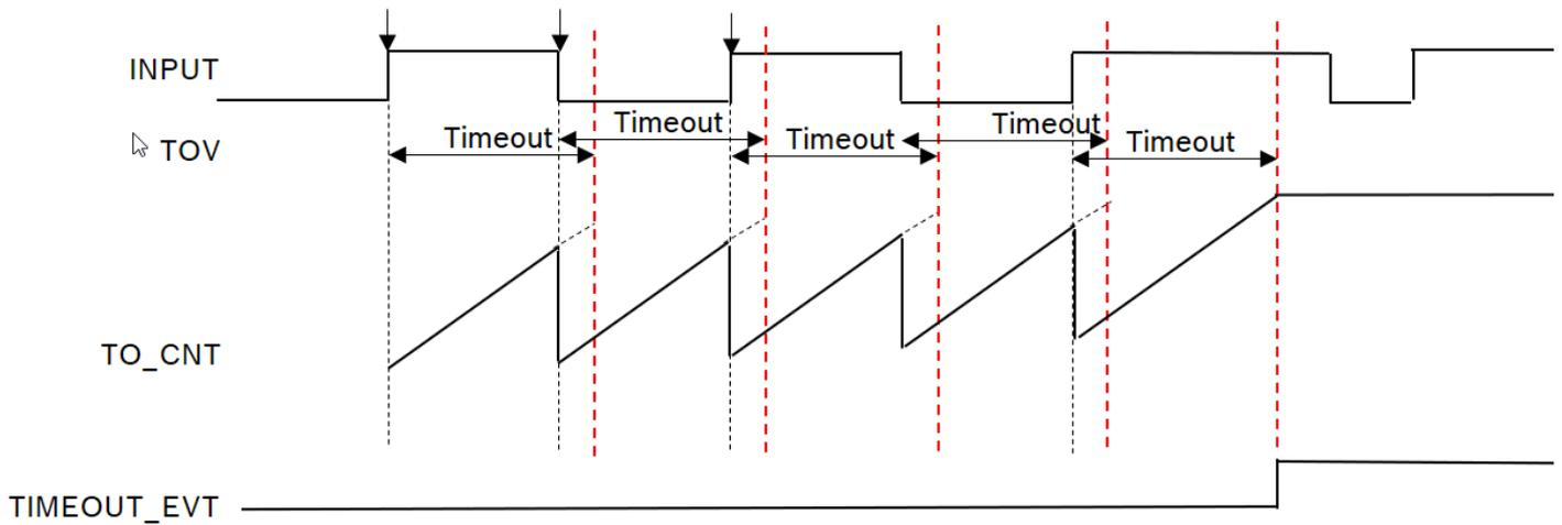
**Figure 1.3: Timeout detection for both edges (unique value for TOV)**
