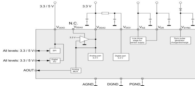
The ASIC operation voltages are V<sub>DIO</sub>, V<sub>DAA5</sub>, V<sub>D3</sub>, V<sub>ER</sub>, and V<sub>SYNC</sub>. V<sub>DAA5</sub> is the 3.3 V power supply for the analog ASIC part and V<sub>D3</sub> is the 3.3 V power supply for the digital ASIC part (clock driven). V<sub>DIO</sub> is the 3.3 V / 5.0 V power supply for the SPI interface and the digital I/O pins.
