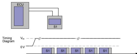
In the synchronous PSI5-S operation, the sensor can transmit a single data word after the sync pulse shifted into time slot 1. Depending on the sensor up to 4 data words can be transmitted using the time slots 1 to 4 according PSI5 specification.
