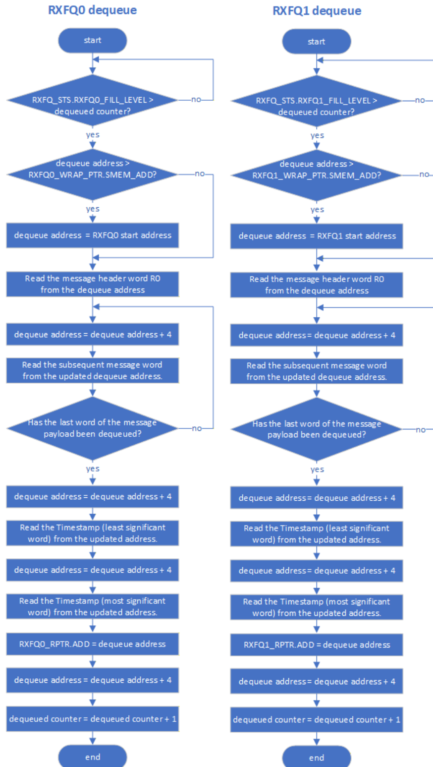
Figure 7 : Dequeue flow diagram for RXFQ0/1
