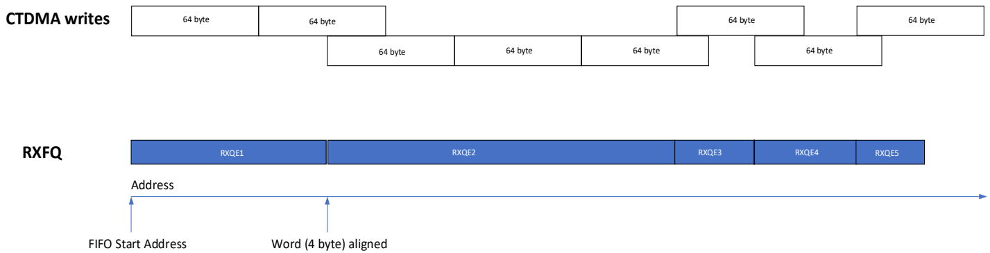
Figure 23. CAN message storage in SMEM (RXFQ)
